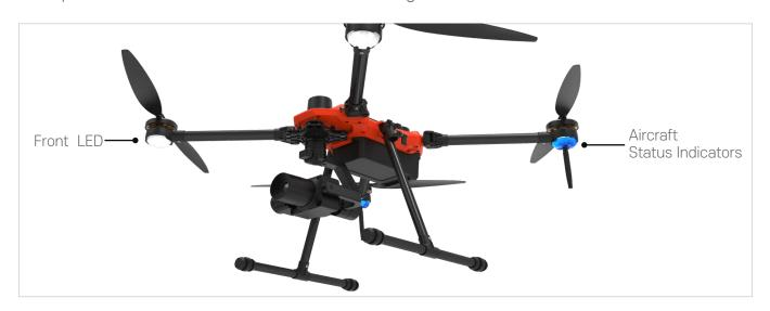
The Front LEDs show the orientation of the aircraft. The Front LEDs glow solid white when the aircraft is turned on to indicate the front (or nose) of the aircraft. The Aircraft Status Indicators communicate the system status of the flight controller. Refer to the table below for more information about the Aircraft Status Indicators.
